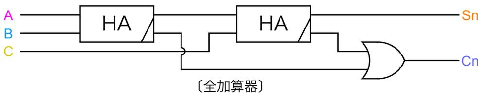
$$S_n = A * B * C + \bar{A} * \bar{B} * C + \bar{A} * B * \bar{C} + A * \bar{B} * \bar{C}$$
