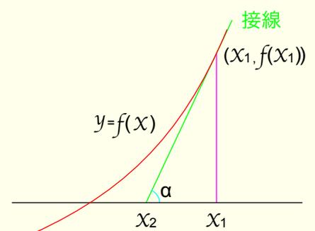
$$\begin{aligned} \tan \alpha &= f'(x_1) \\ &= \frac{f(x_1)}{x_1 - x_2} \\ \therefore x_2 &= x_1 - \frac{f(x_1)}{f'(x_1)} \\ &\text{一般的に } x_1 \text{ なる初期値より} \\ x_{i+1} &= x_i - \frac{f(x_i)}{f'(x_i)} \\ &\text{を繰り返せば近似値の精度向上} \end{aligned}$$
